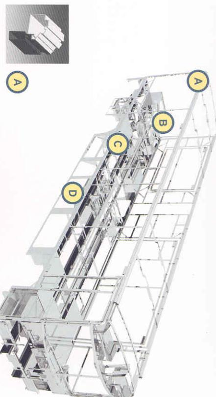
**SUPERSTRUCTURE** is the term given to Winnebago Industries' structural motor home design and construction. Rather than a single component, it is the culmination of design integration that incorporates steel and aluminum substructures; composite-design laminated floor risers; interlocking joint technology; and Thermo-Panels® floor, roof and sidewalls to form a high-strength, durable vehicle body.
