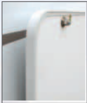
Exterior storage doors are extra thick with radius corners for added protection and durability.
