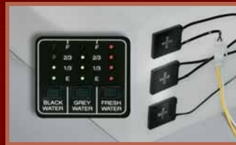
WEB TRUELEVEL® holding-tank monitoring system uses sonar technology to read liquid levels from outside the tank. There are no probes to corrode or clog, just accurate readings time after time.
