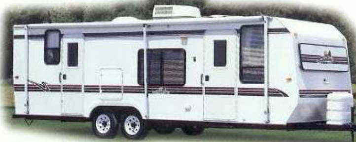
• SE Package - Smooth, seamless white fiberglass exterior w/1/4" offset layered luan backing. Features include: better resale value, easy to keep clean, improved R-value of insulation, aerodynamic shape. SE Package for Solaris models only. (Not available on Solaris SR and Saturn.)
