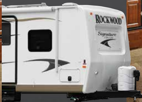
Tinted Bonded Frameless Windows with White Fiberglass (Platinum Package only)
