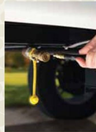
LP gas hook up
