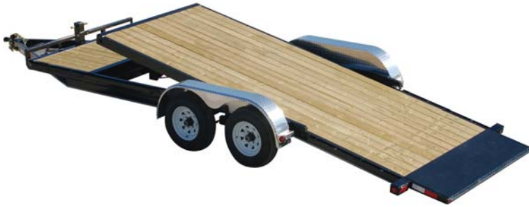
20 ft 5" Channel Tilt (T5) Pictured (4' Stationary Deck + 16' Tilt)
