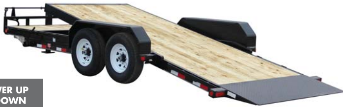
20 ft 6" Channel Tilt (T6) Pictured (4' Stationary Deck + 16' Tilt)
