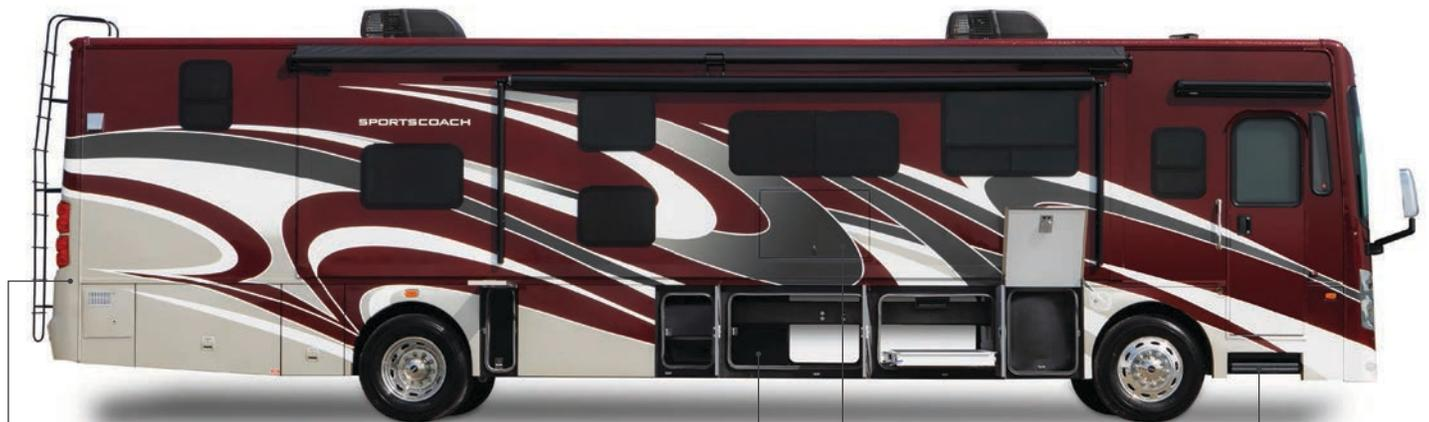
With a 360 horsepower ISB Cummins rear diesel engine and a 6-speed Allison 3,000 MH automatic transmission, Sportscoach gets 800 lbs./ft. of torque and has a 10,000 pound towing capacity.
