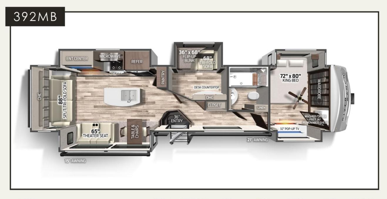
HITCH BLACK OVERALL EXT. HEIGHT EXT. FRESH GREY AWNING (w/AC) WATER WEIGHT UVW **GVWR** CCC LENGTH WIDTH WATER WATER SIZE 42' 0" 2,455 Lb. 14,844 Lb. 17,999 Lb. 3,155 13' 6" 101" 75 Gal. 39 Gal. 21' & 15' 78 Gal.
