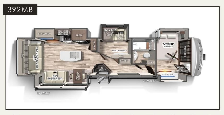
HITCH WEIGHT BLACK WATER OVERALL EXT. HEIGHT EXT. FRESH GREY AWNING UVW GVWR CCC LENGTH (w/AC) WIDTH WATER WATER SIZE 42' 0" 13' 6" 2,455 Lb. 3,155 101" 75 Gal. 39 Gal. 14,844 Lb. 17,999 Lb. 78 Gal. 21' & 15'
