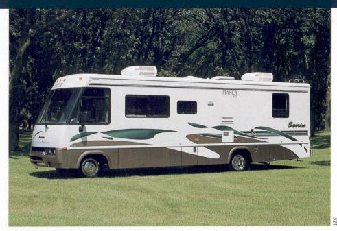
While our smooth, one-piece fiberglass exterior is certainly good looking, the advantages of this design go far beyond mere aesthetics. This outer skin is laminated to a rigid lauan backing material. A layer of block foam insulation is applied over this backing material. This insulation is then routed to embed the welded aluminum framework. The result is one of the most durable, rigid sidewall constructions in the industry.
