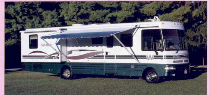
L35U An innovative awning rail with built-in gutter keeps things dry by channeling water to the front and rear of the coach. And unlike rubber roofs, the one-piece, seamless fiberglass roof resists tearing, fading, chalking and deterioration.
