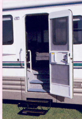
L34Y The entrance features sturdy interior and exterior assist handles. The auxiliary battery disconnect switch is located inside the door. The KeyOne™ system lets you open most doors with just one key.
