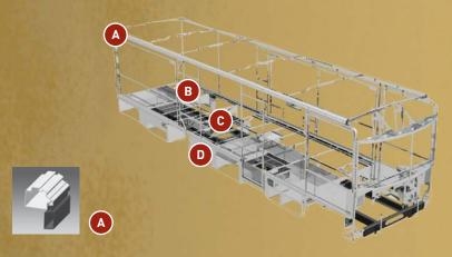
SUPERSTRUCTURE® is the term given to Winnebago Industries' structural motor home design and construction. Rather than a single component, it is the culmination of design integration that incorporates steel and aluminum substructures; welded tubular steel floor risers; interlocking joint technology; and Thermo-Panel® floor, roof and sidewalls to form a high-strength, durable vehicle body.
