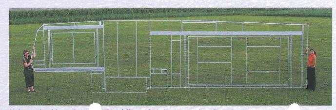
Light yet durable — Sprint HP's" fully welded aluminum sidewall.
