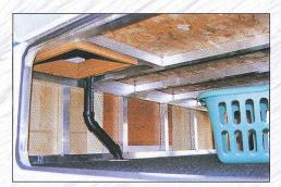
Welded aluminum supports in all raised-bath fifth wheel decks provide strength and rigidity in all critical high-stress pas.
