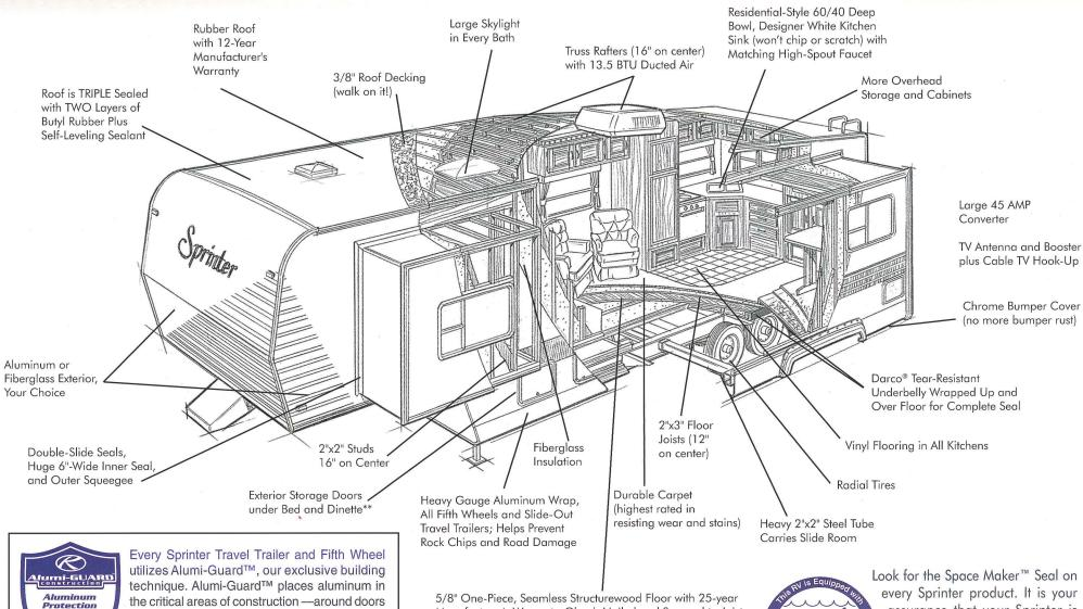
the critical areas of construction —around doors and exterior storage compartments, providing the protection that only aluminum can offer. Alumi-Guard™ extends the life of your Sprinter by protecting these areas from the damaging effects
