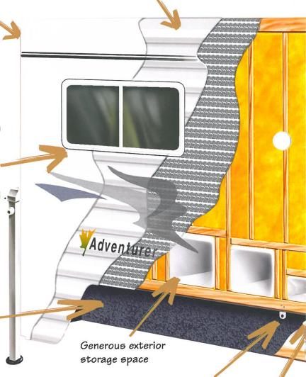
Tie-down brackets are bolted to the main wall and wing wall for extra reinforcement and strength
