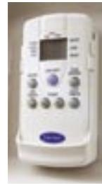
Challenger's Carrier® roof-mounted air conditioner is run by this programmable remote-control thermostat.
