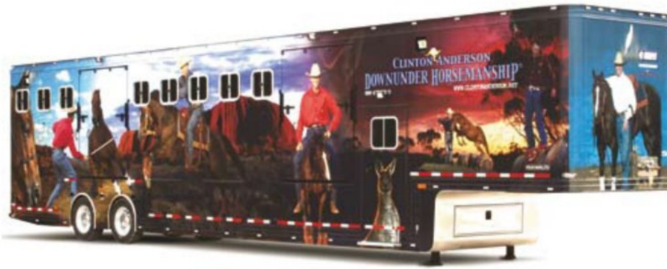
Custom 53' horse trailer This trailer custom built for Clinton Anderson accommodates 12 horses along with storage for tack, displays and materials for clinics and demonstrations. It also includes two side ramps, a rear ramp and a wireless camera for monitoring the horses!
