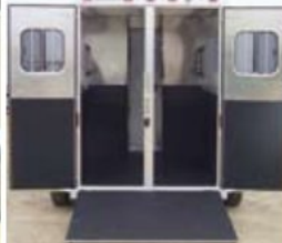
Optional full-width ramp behind doors - versatility for easier unloading
