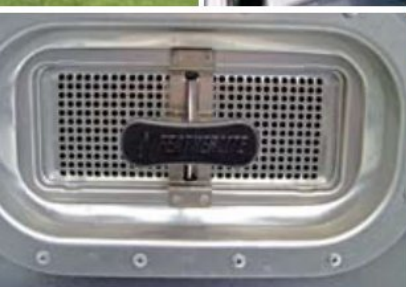
2-way roof vents on most models - one per horse
