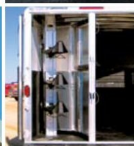
Solid mount adjustable saddle racks
