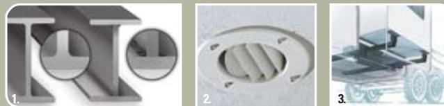
1. (Left) End view of Jayco's I-Class™ structural steel chassis frame. (Right) End view of the welded I-beam frame used by many competitors that is subject to warping.
