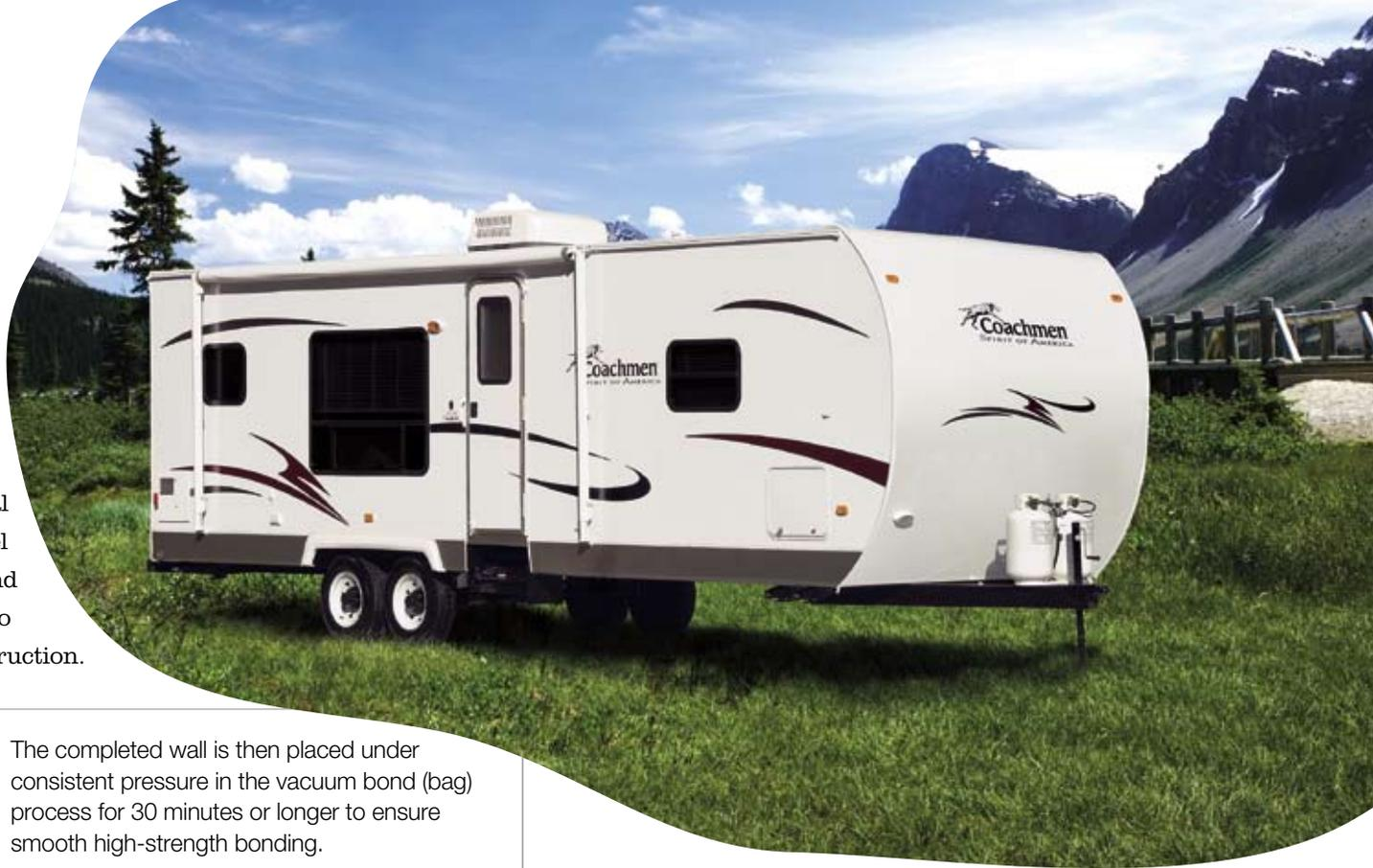
High strength urethane adhesive, bonds a smooth fiberglass sheet to a lauan backing for the exterior wall. The walls are bonded with urethane to a welded aluminum frame that is filled with rigid polystyrene insulation. Finally, an interior panel is glued to the inside of the wall.
