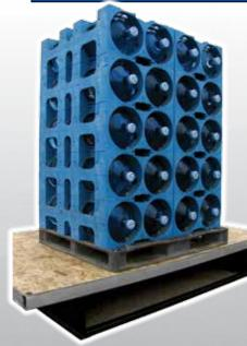
Heartland's laminated floor construction easily supported over 1,800 lbs. of water jugs in one spot - resulting in less flex!!
