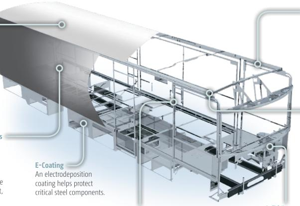
**Embedded Steel** Metal substructures embedded into the sidewall provide solid attachment points to keep cabinets and appliances mounted securely in place.
