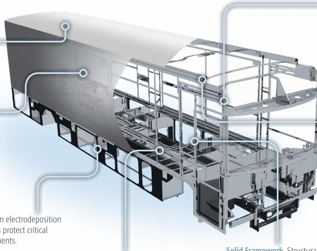
**Laser-Cut Tubing** Precision laser cutters create precise joints in structural steel that are stronger and require less welding.
