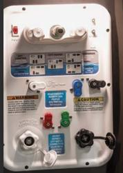
**Heated Water Convenience Center** Includes black tank flush, power fresh tank water fill, winterizing system and outside shower.
