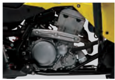
398cm³ liquid-cooled engine
