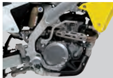
Lightweight four-valve, DOHC engine
