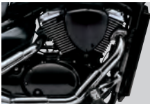
Liquid-cooled, 45-degree V-Twin engine
