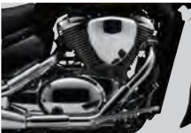
Liquid-cooled 45-degree V-Twin engine
