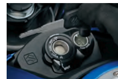
Suzuki Easy Start System, with Shutter-Key Lock
