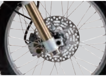
250mm (9.8in) front disc brake
