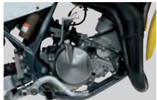
84.7cm 3 2-stroke engine
