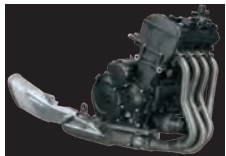
999cm 3 liquid-cooled engine
