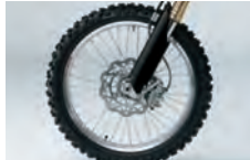
Lightweight front brake caliper and Dunlop MX52 series tires
