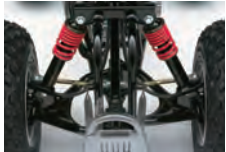
Single A-arm front suspension
