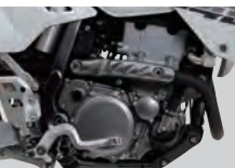
Liquid-cooled, DOHC engine
