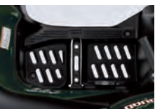
Full floorboards with drain holes
