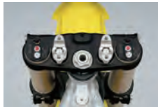
PSF2 front fork (KYB's Pneumatic Spring Fork)
