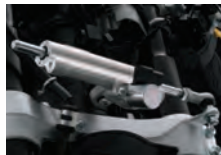
Electronically controlled steering damper
