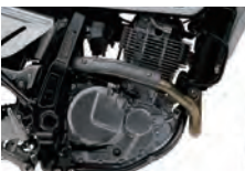
Air-cooled, SOHC engine
