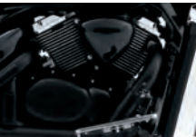
1462 cm³ liquid-cooled V-Twin engine
