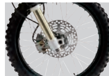
250mm (9.8 in) front disc brake
