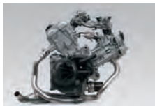
645cm 3 liquid-cooled, DOHC 90-degree V-Twin engine
