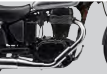
652cm³ Single cylinder engine
