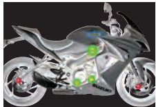
Suzuki Traction Control System (STCS)
