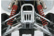
Double-wishbone front suspension
