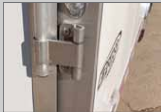
ALUMINUM BAR LOCKS WITH STAINLESS STEEL FASTENERS
