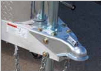
DOUBLE TUBE A FRAMES WITH STEEL COUPLER
