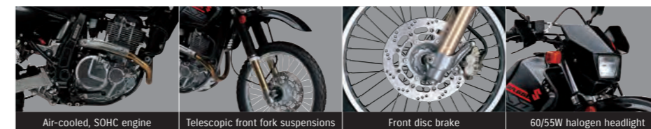
Air-cooled, SOHC engine Telescopic front fork suspensions Front disc brake 60/55W halogen headlight
