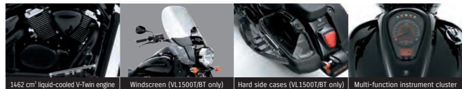
1462 cm 3 liquid-cooled V-Twin engine Windscreen (VL1500T/BT only) Hard side cases (VL1500T/BT only) Multi-function instrument cluster
