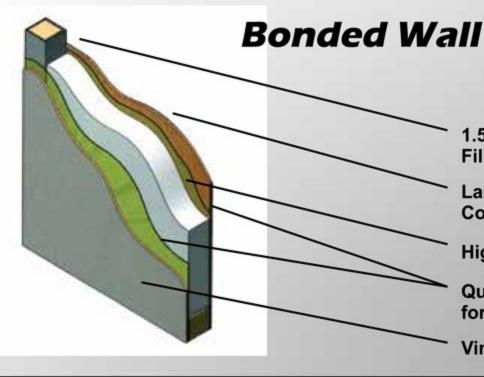
1.5 x 1.5 Welded Aluminum Tube Filled with Lumber for Better Screw Retention
