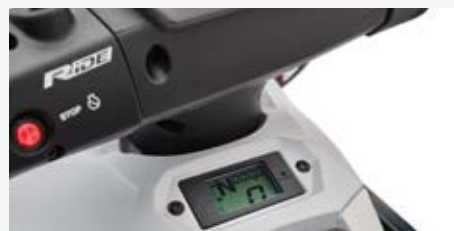
RiDE system (Reverse with Intuitive Deceleration Electronics)
