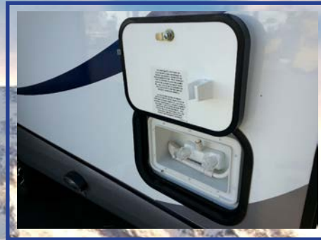
Exterior Shower Insulated by 1" Thick Thermal Insulated Luggage Door
