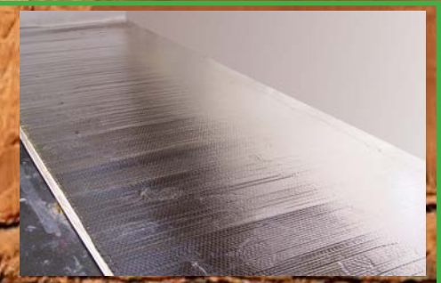
Reflective Insulation Blanket Applied to Roof, Slide-Out Floor, Entire Underbelly, Additional Wrap Around Holding Tanks
