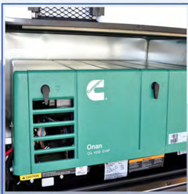
Cummins Onan 4000 Watt Gas Generator
