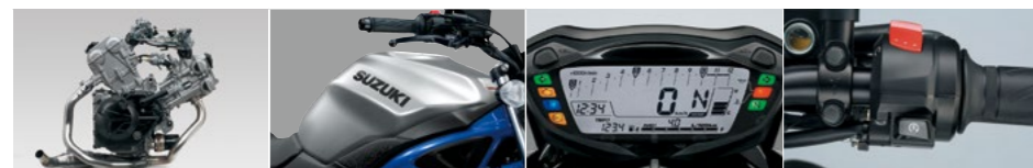
645cm 3 liquid-cooled, DOHC 90-degree V-Twin engine 14.5-litre capacity fuel tank Multi-Function, Full LCD Instrument Cluster Suzuki Easy Start System
