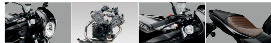
Stylish Slotted Headlight Cowling 645cm 3 liquid-cooled, DOHC 90-degree V-Twin engine Clip-on Handlebars Tuck-and-Roll Seat
