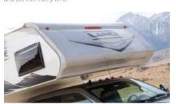
TPO Front Nose Cap - Protects your camper from debris and leaks while reducing drag and increasing fuel economy.
