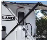
Rear Awning – Provides protection from the elements over the rear of your camper. Is model specific in either electric or manual operation, N/A 1172
