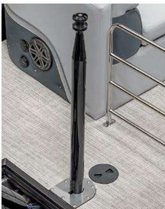
SKI TOW PYLON
