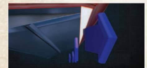
Reverse chines along hull sides to deflect spray
