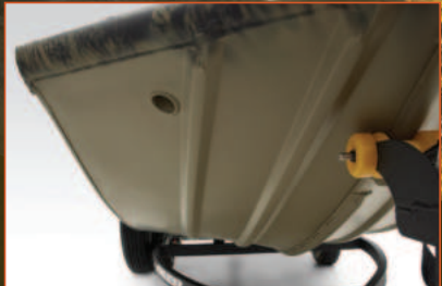
Heavy-Duty Icebreaker Keel, .125" construction, and Sch. 40 Bull-Nose Bow
