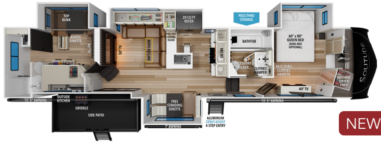
414LJM UVW 1 19,000 HITCH 1 3,100 GVWR 23,500 LENGTH 2 42' 10" HEIGHT 3 13' 5" CAPACITY 83 159 106
