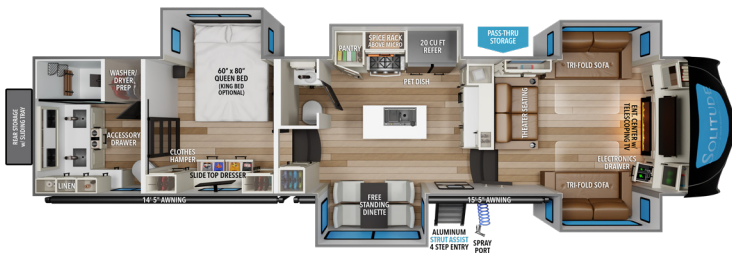
380FL UVW 1 15,000 HITCH 1 3,052 GVWR 19,000 LENGTH 2 41' 4" HEIGHT 3 13' 5" CAPACITY 83 106 106
