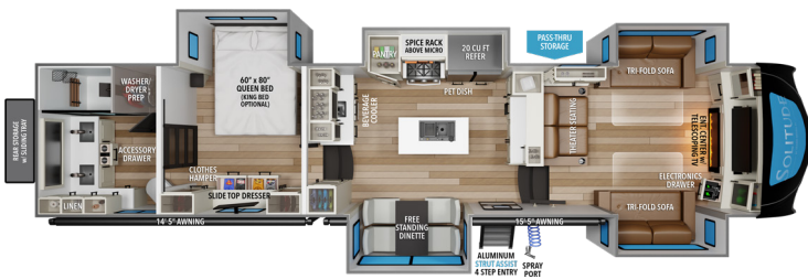
382WB UVW 1 15,200 HITCH 1 2,930 GVWR 19,000 LENGTH 2 41' 4" HEIGHT 3 13' 5" CAPACITY 83 106 53
