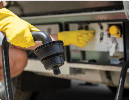
Macerator Sewage Discharge With Manual Disconnect
