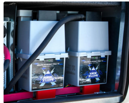
Additional Smart Lithium Battery 270-Ah 12-V with Internal Heating System (540-Ah total)
