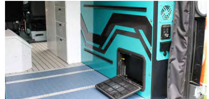
8.4 kWh 51V Lithionics® Power System
