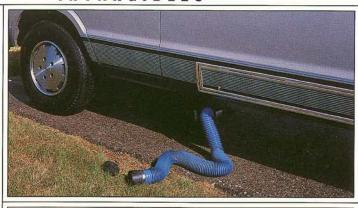
18. Patented 'Dura-Drain' sewage hose system provides a permanently attached built-in sewage hose that eliminates sewage hose handling and storage inconvenience.
