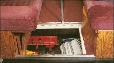
14. Additional storage space is supplied within our unique storage trunk (optional) located beneath the floor at the rear of the unit.
