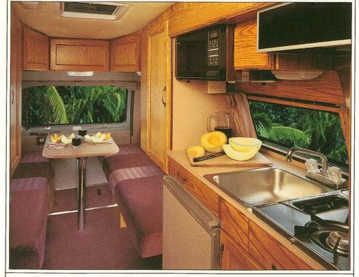
16. Fully equipped galley that features a 'Dometic' 3.0 cu. ft. 3-way refrigerator, variable intensity microwave oven, LP gas stove, exhaust fan, sink, monitor panel and LP gas
