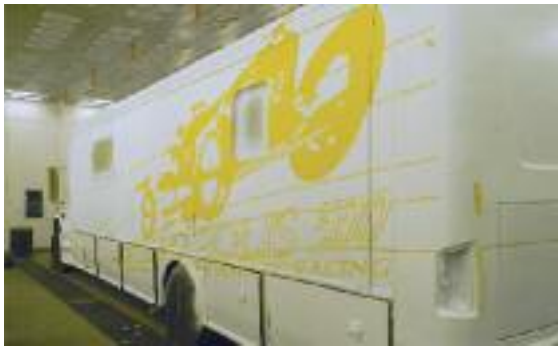
Digitally plotted, spray mask is carefully applied
