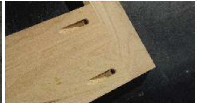
Pocket screws for structural integrity
