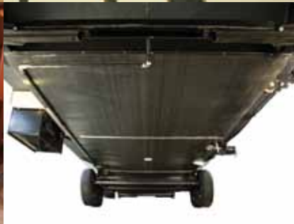
Enclosed underbelly protects trailer components as well as increasing aerodynamics (Ultra Lite only)
