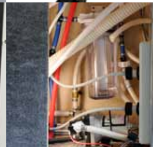
Outside Antifreeze Inlet with Easy Access to Water Pump in Storage Compartment for Convenient Winterizing. (Std.)
