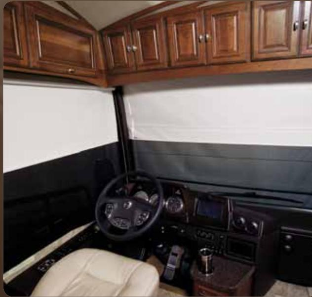
**Power Shade** The powered MCD American Duo front roller shade features a separate blackout and solar screen. It also functions as a sun screen.
